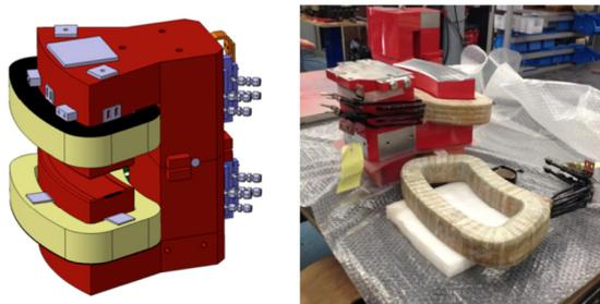
Figure 3: a) Drawn and b) Manufactured dipole.
