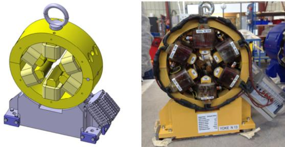
Figure 6: a) Drawn and b) Manufactured sextupole.
