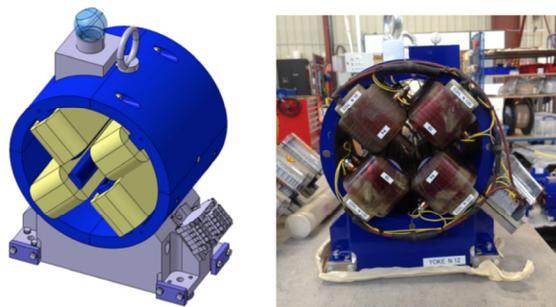
Figure 5: a) Drawn and b) Manufactured quadrupole.
