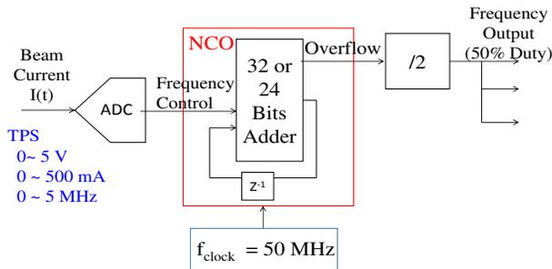
Figure 3: Functional block diagram of a VFC.
