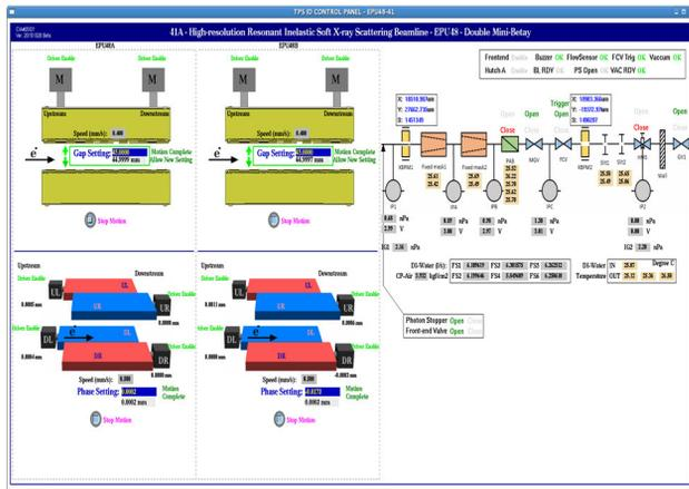
Figure 7: GUI of a double EPU48 installed at a long straight section of TPS.
