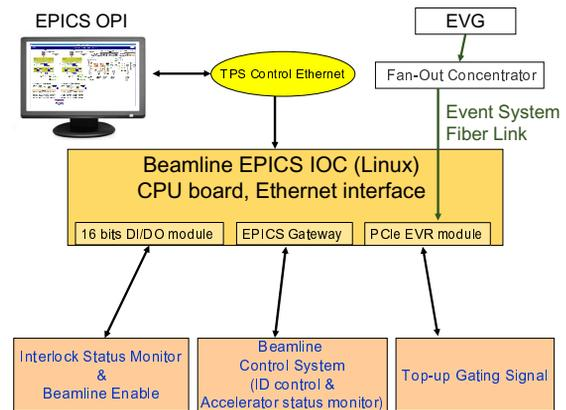
Figure 1: Architecture of a beamline EPICS IOC.
