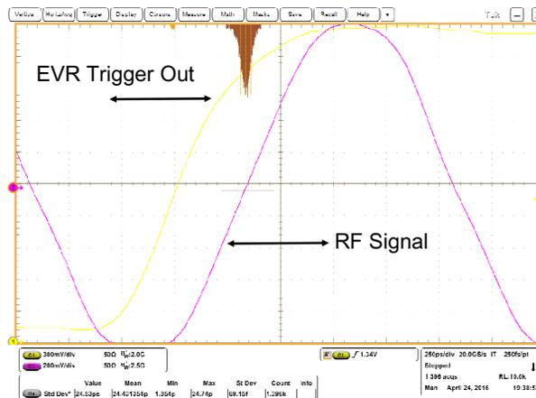
Figure 5: Jitter of PCIe-EVR-300 TTL output relative to the RF clock.
