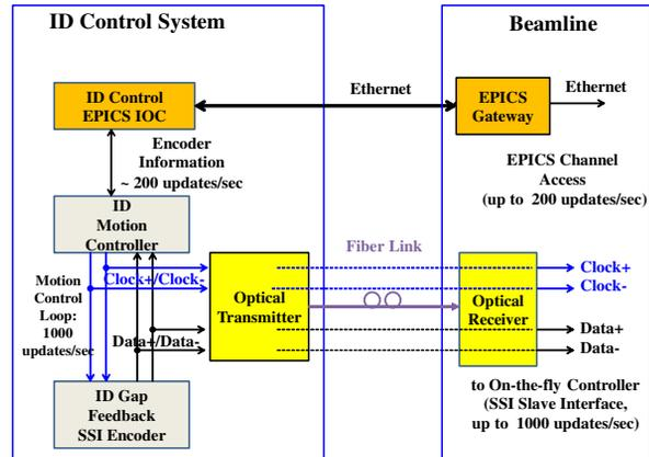
Figure 8: Support of insertion devices for on-the-fly or continuous scan
