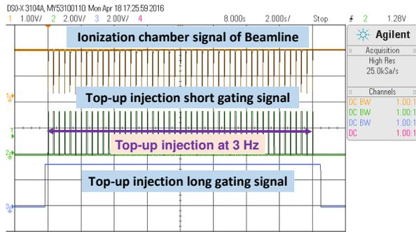
Figure 6: Top-up injection short gating and long gating signals versus ionization-chamber signal of beamline during top-up injection.
