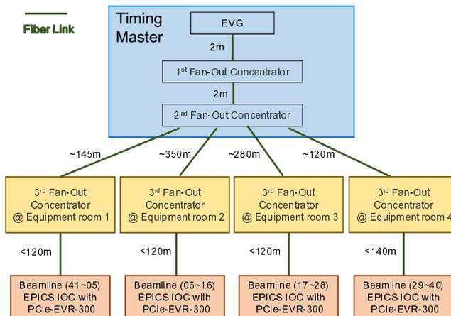
Figure 4: Configuration of an event system link for a beamline
