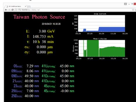
Figure 2: Web-based machine status broadcasting of TPS.
