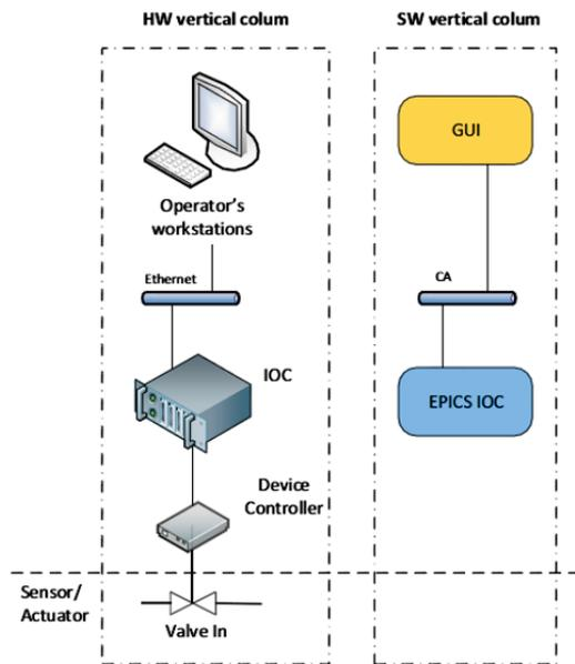
Figure 1: Vertical Column concept. Hardware and Software models comparison on the left.
