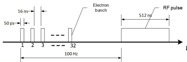
Figure 4: 32 Bunches train temporal structure.
