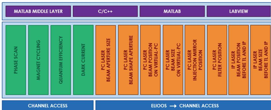
Figure 2: General purpose tools; in green electron beam tools, while in orange laser and gamma beam tools. The first bunch of tools get information directly from the EPICS CA while the second bunch uses data collected from the laser systems CS, called ELIOOS, which shares data on the EPICS CA.
