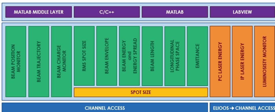
Figure 3: Beam Diagnostics tools; in green electron beam tools, while in orange laser and gamma beam tools. The first bunch of tools get information directly from the EPICS CA while the second bunch uses data collected from the laser systems CS, called ELIOOS, which shares data on the EPICS CA.
