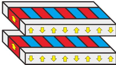
Figure 2: Force cancellation with monolithic repulsive magnets placed aside of the main magnets.
