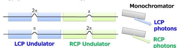
Figure 5: Fast helicity switching by spectrum splitting.
