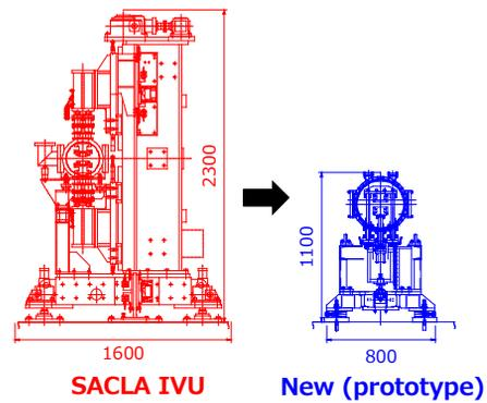
Figure 3: Left: Cross-sectional view of the SACLA IVU. Right: Prototype of the lightweight and compact frame.
