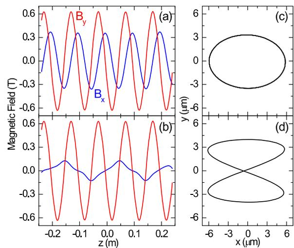
Figure 4: Measured magnetic field distributions (a,b) and computed electron trajectory (c,d) of the helical-8 undulator prototype.
