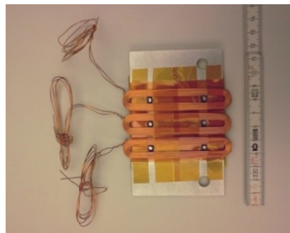
Figure 6: 3-coils set for horizontal and vertical beam steering. One unit is mounted above, one below the beam.
