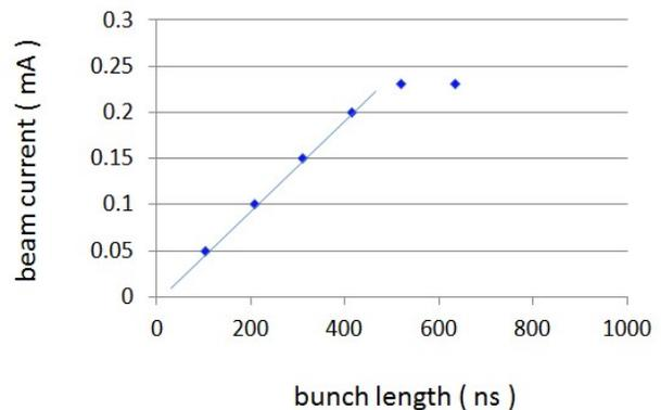
Figure 8: Typical measurement of the booster beam current as a function of the length of bunch train applied.
