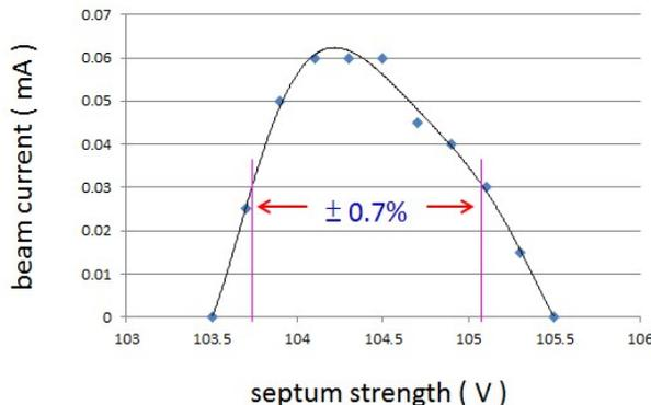
Figure 5: The tuning range of the injection septum in a typical top-up operation.
