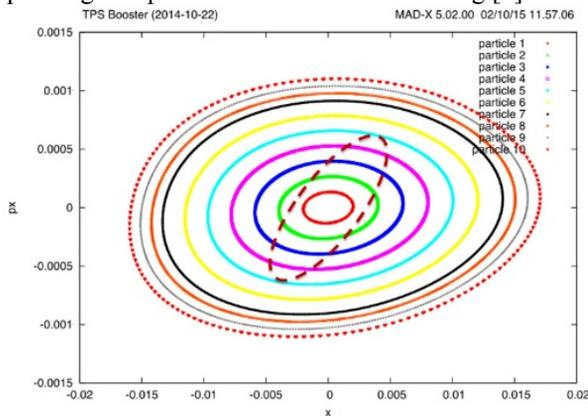
Figure 7: The phase space particle tracking of the designed TPS booster observed at the injection kicker location. The operational horizontal phase space given in Fig. 6 is depicted here, i.e. the brown dash line circled region, for comparison purpose.
