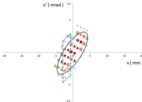
Figure 6: The measured horizontal phase space acceptance of the TPS booster at injection kicker. The green dash line circled region is depicted here for comparison purpose based on an independent measurement result given in [6].
