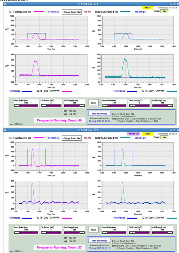
Figure 2: The transfer rate (ICT2/ICT1) of LTB has been improved up to ~85%. The upper one is the multi-bunch mode and the lower is the single-bunch mode.
