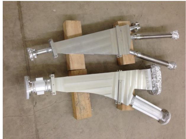
Figure 1: The TPS LTB bending chambers are arranged in parallel for comparison purpose. The upper chamber was built with small entrance/exit apertures while the lower newly build chamber is equipped with wider entrance/exit channels.
