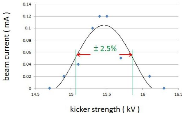
Figure 4: The tuning range of the injection kicker in a typical top-up operation.
