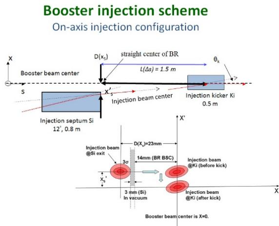
Figure 3: The LTB-to-booster beam injection scheme and its corresponding horizontal phase space evolution.
