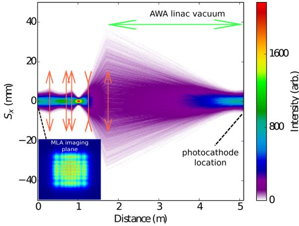
Figure 2: Ray tracing of a five-lens transport capable of imaging the homogenized beam to the photocathode (this system was built at AWA). The inset shows a  $8 \times 8$  simulated through the MLA using srw [6] (bottom left).
