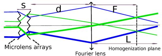
Figure 1: Schematics of the microlens array configuration. Initial incoherence in the beam becomes evenly distributed at the homogenization plane.
