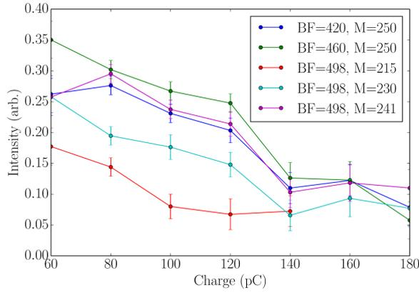
Figure 5: First harmonic amplitude as a function of charge for different solenoid settings at 8 MeV.
