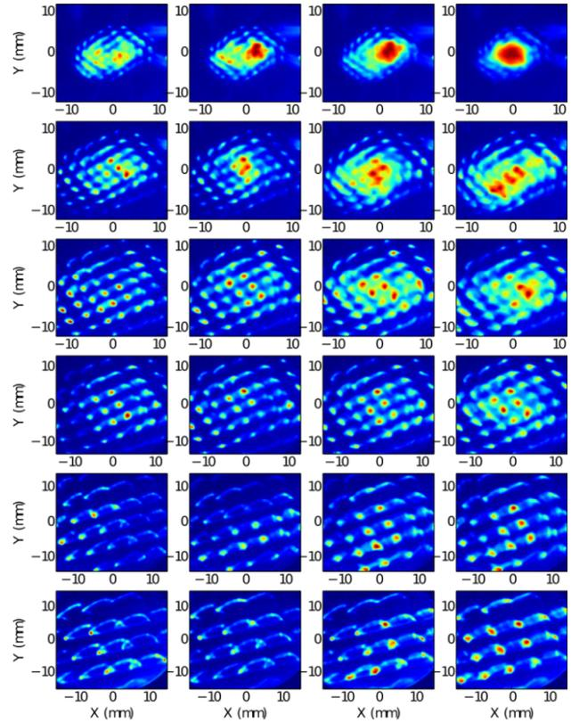
Figure 6: False color 8 MeV electron beam patterns for various matching solenoid current setting and charge. Left to right:  $Q=60\text{pC}$ ,  $80\text{pC}$ ,  $100\text{pC}$ ,  $120\text{pC}$ . Top to bottom:  $M=215\text{A}$ ,  $230\text{A}$ ,  $241\text{A}$ ,  $255\text{A}$ ,  $270\text{A}$ ,  $290\text{A}$  and  $\text{BF}=498\text{A}$ .
