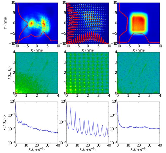
Figure 3: Measured UV laser without MLA (left column) and with MLA setup to produce beamlets (middle column) or as a homogenizer (right column). The upper, middle, and lower rows respectively correspond to the laser transverse density distribution, its 2D FFT, and the projected spectrum along the horizontal frequency  $k_x$ .
