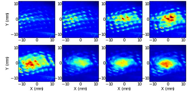
Figure 7: False color 50 MeV electron beam patterns for various charges. From left to right and top to bottom:  $Q=60\text{pC}$ ,  $100\text{pC}$ ,  $200\text{pC}$ ,  $300\text{pC}$ ,  $400\text{pC}$ ,  $500\text{pC}$ ,  $600\text{pC}$ ,  $700\text{pC}$ .
