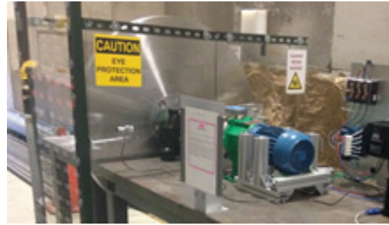
Figure 1: Picture showing a modified pump with magnetic torque coupler driving a solid aluminum wheel.
