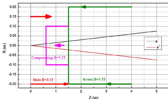
Figure 7: Solenoid compensating layout.
