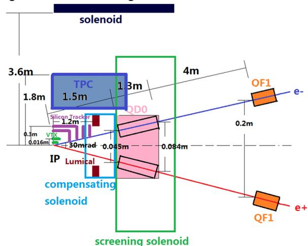
Figure 1: IR layout of CEPC partial double ring.
