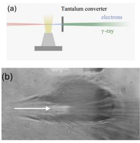
Figure 4: (a) Illustration of the setup; (b) Shadowgraphic image of plasma channel [22].
