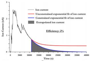
Figure 1: Laser ionized <sup>76</sup>Ge ion current against time during the efficiency measurement [4].
