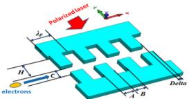
Figure 2: Schematic drawing of a dual-grating structure.
