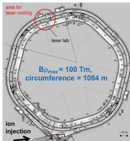
Figure 1: The laser cooling facility at the SIS100.
