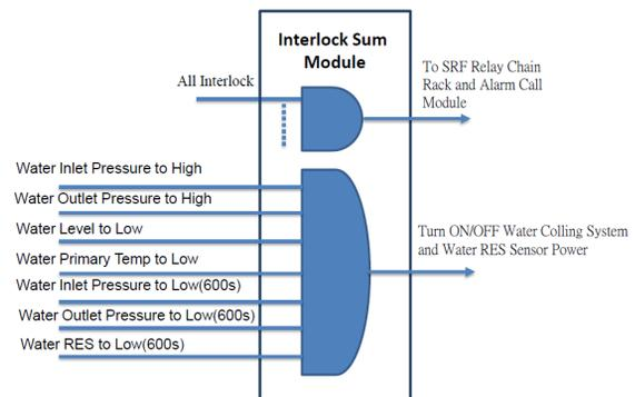
Figure 9: System protection logic.
