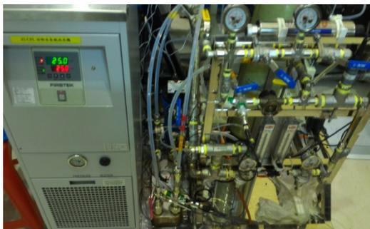
Figure 4: Cooler and water manifold of the CPL water-cooling system.
