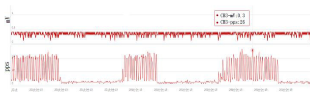
Figure 8: A one-day trend of partial discharge monitored by the installed system at the position shown in figure 7.
