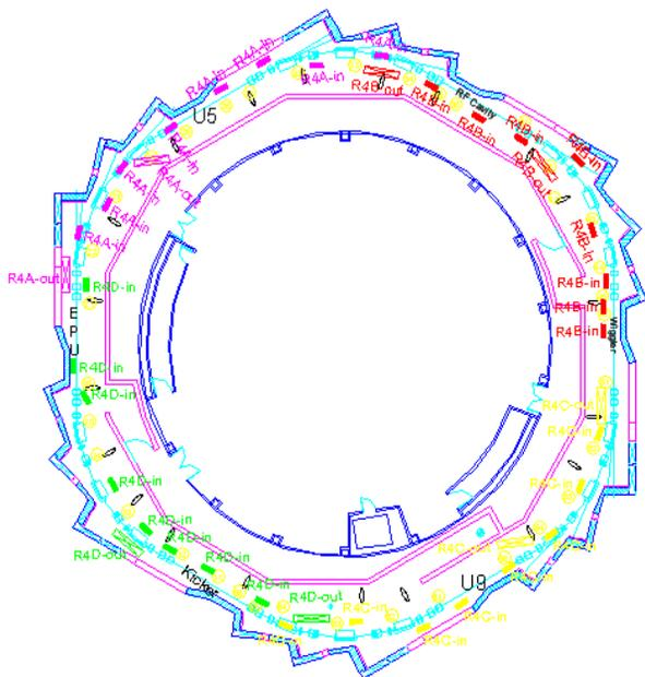
Figure 2: Air conditioning ventilation inlet and outlet distribution in the TLS storage ring tunnel.
