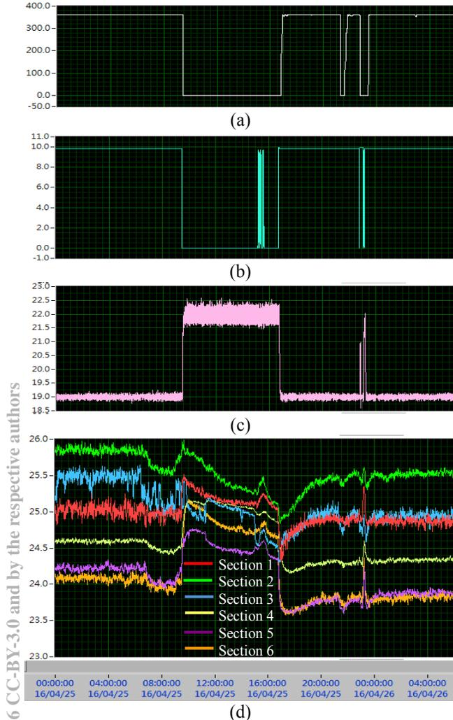
Figure 5: Histories of beam current (a), status of dipole magnets (b), supplied air temperature (c) and air temperature in 6 sections of TLS (d).
