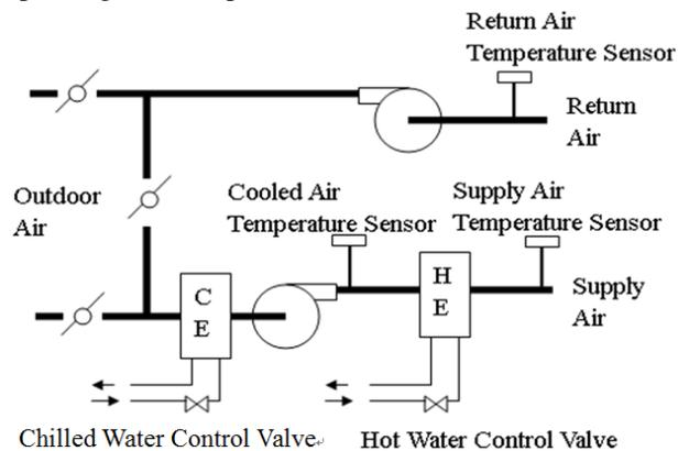
Figure 1: Control system of the AHU for TPS tunnel.
