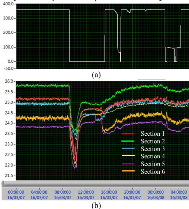
Figure 4: Beam current (a) and air temperature histories in 6 sections of TLS (b).
