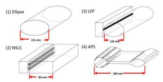
Figure 5: Simplified 3D models of the interior volumes of four aluminum vacuum chambers for use in MolFlow+.
