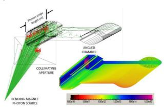
Figure 1: PSD measurement ray trace created in SynRad (left) with calculated spatial photon flux densities in log scale and units of photons/cm<sup>2</sup>/s (right).
