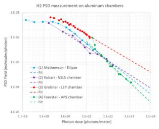
Figure 6: Comparison of  $H_2$  PSD measurements and power law curves fit to the data for the four aluminum vacuum chambers in the study.
