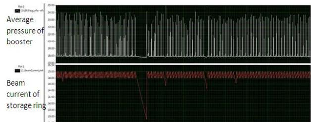
Figure 4: Average pressure of the booster ramped up when the storage ring was in the top-up mode at 150mA
