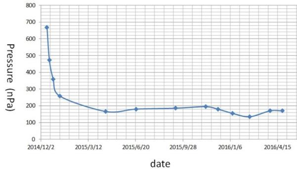
Figure 3: Decreasing trend of average pressure with no electron beam stored in the booster ring
