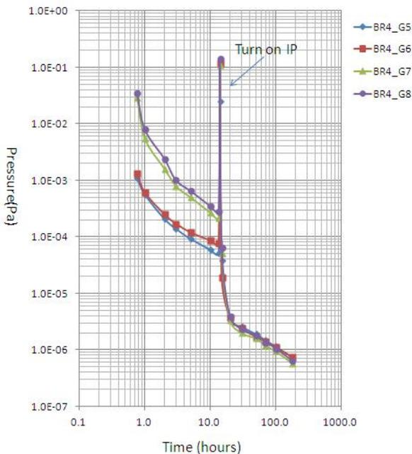
Figure 2: Pumping curve for one section of the TPS booster vacuum system
