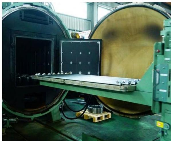
Figure 1: The SUS304 elliptical tube is transported into a vacuum furnace of length 2.2 m.
