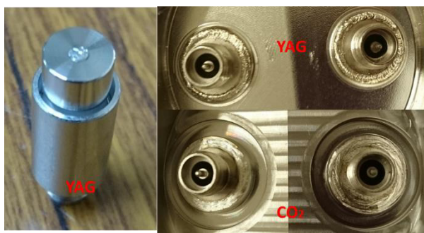
Fig 6: Welding beads of YAG and CO 2 LBW respectively
