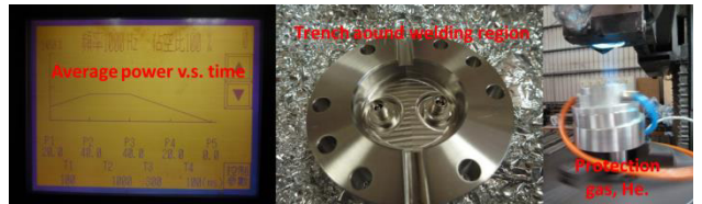
Fig 5: Jointing a feedthrough into a flange with CO 2 LBW
