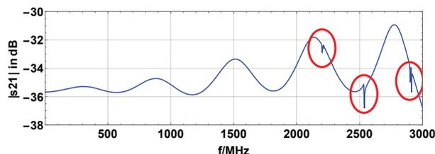
Figure 2: Magnitude of transmission S-parameter signal  $S_{21}$  of cavity modes observed with the wire method in frequency domain. Data from 2-convolution RF-fingers.
