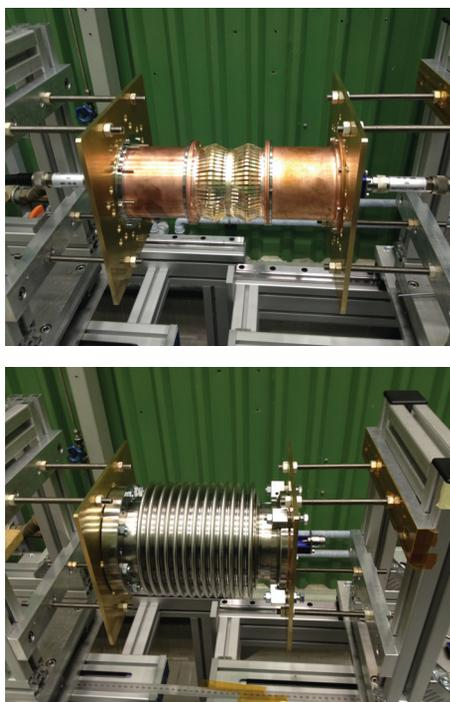
Figure 3: Top: Picture of the RF-fingers with 2-convolutions, bottom: RF-fingers in outer bellows on measurement bench.
