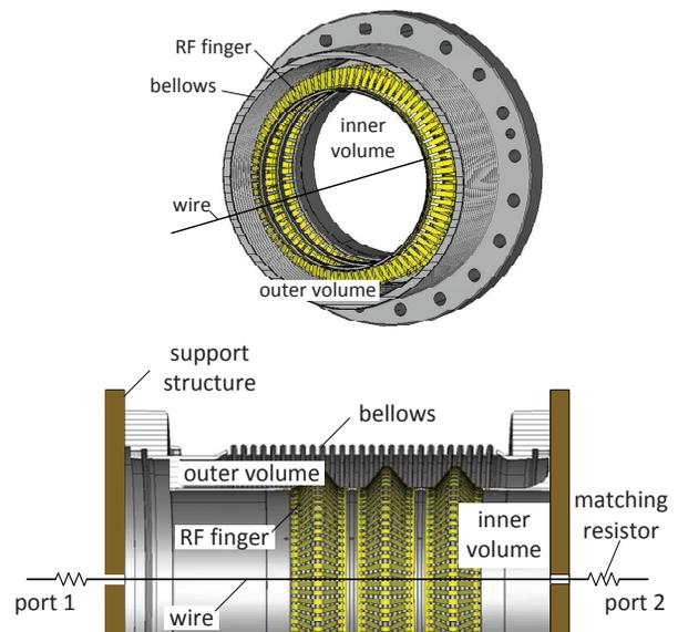
Figure 1: Top: transverse cross-section, and bottom: longitudinal cross-section of nested coaxial structure consisting of outer (stainless steel) bellows and (copper-beryllium) 3-convolution RF-fingers with centered measurement wire.
