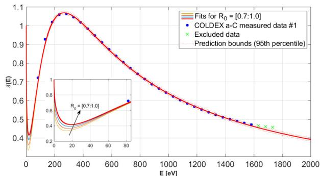
Figure 4: The a-C SEY curve fitted model.
