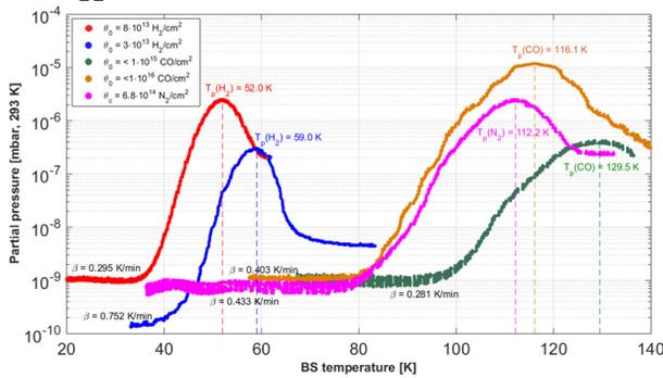
Figure 1: TDS for  $H_2$ ,  $N_2$  and CO measured for a-C coating as a function of  $\theta_0$  and  $\beta$ .
