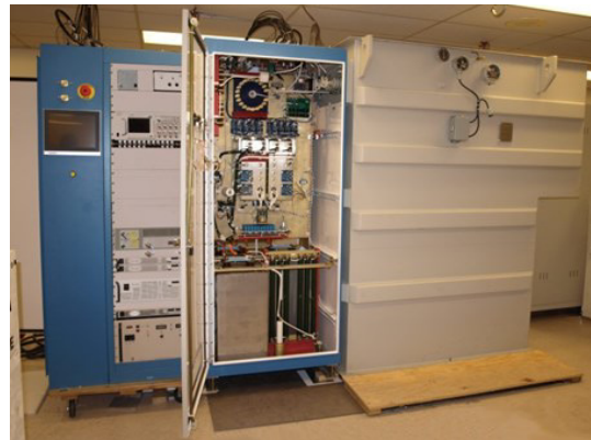
Figure 1: DTI's prototype solid -state ESS-class klystron modulator, developed under a DOE SBIR grant. This design is optimized for long pulse operation with highest possible reliability and availability required for particle accelerator user facilities and test stands.
