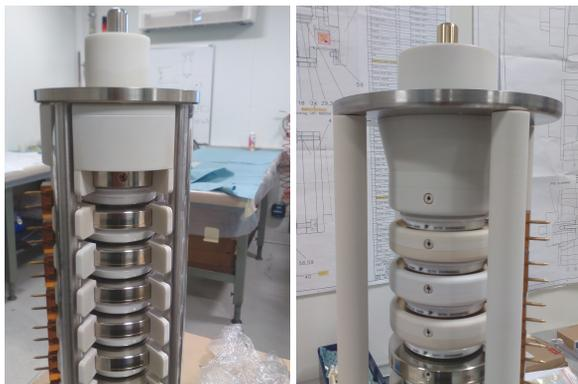
Figure 3: GTO stacks: (left) installed after LS1 and (right) prototype of the new design.
