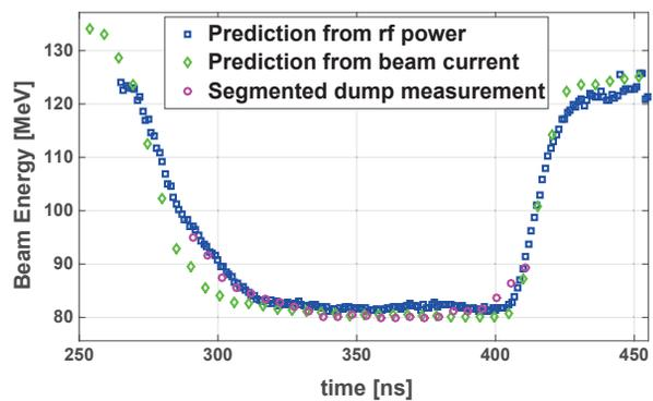
Figure 2: Comparison of measured RF power with predictions from the measured beam intensity and drive beam energy loss.
