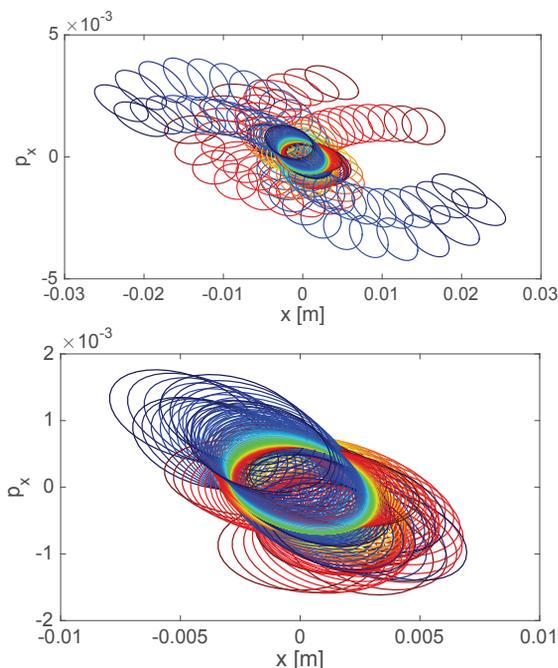
Figure 1: Comparison of beam phase space after CR for old (top) and new (bottom) DL optics.
