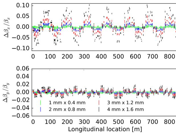
Figure 1: Simulated  $\beta$ -beating of single particles tracked through the nominal lattice with the nominal model used for reconstruction by N-BPM method, with transverse displacement at  $\beta_x = 36$  m and  $\beta_y = 6$  m as shown in the legend (notation: horizontal x vertical).
