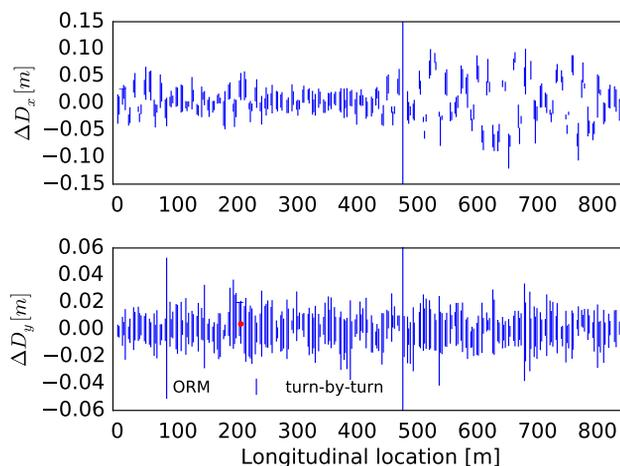
Figure 4: Dispersion deviation from the nominal model obtained from ORM and turn-by-turn data.
