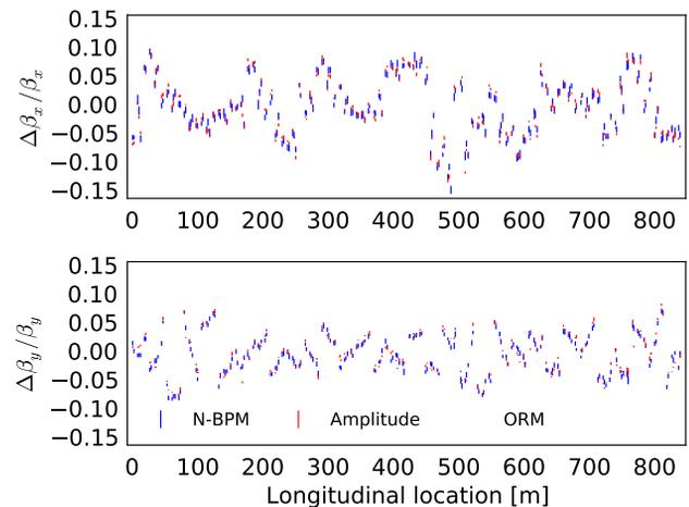
Figure 2: Measured  $\beta$ -beating with respect to the nominal model obtained by three different methods: N-BPM, Amplitude and ORM.
