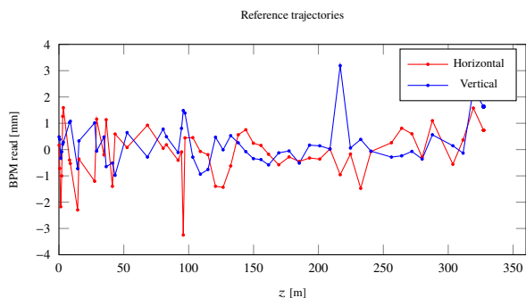
Figure 2: Reference trajectories measured with MEBT_Mag:DCH01 and MEBT_Mag:DCV01 switched off.
