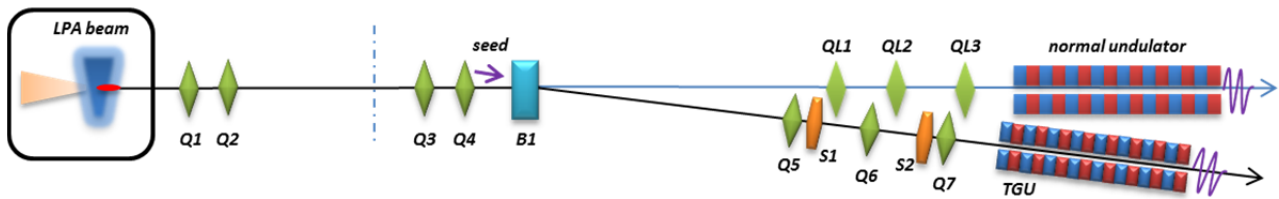
Figure 1: Schematic layout of the beam transport line for the LPA FEL facility in SIOM.
