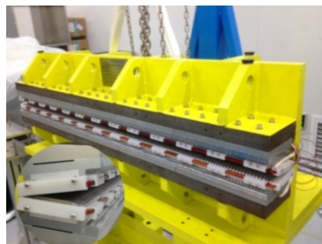
Figure 5: Image of transverse gradient undulator with a canting angle of 7.5 degree designed in SINAP.
