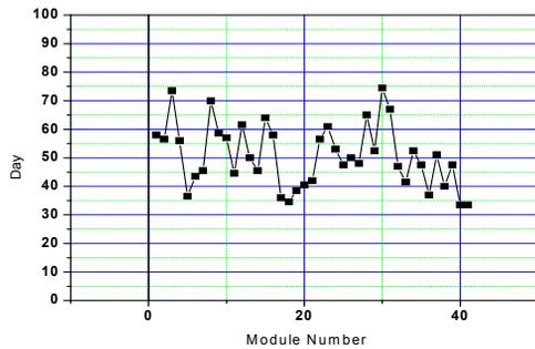
Figure 4: Spent time for conditioning the high power components.
