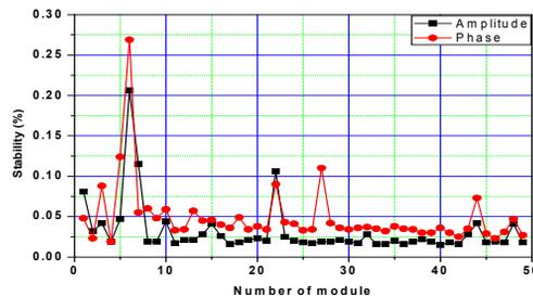
Figure 5: Maximum variations of the amplitudes and the phases of the all modules in the HX linac.
