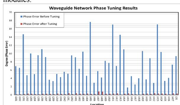
Figure 3: Tuning results of the waveguide networks (Blue bars are the phase error before tuning and red bar phase error after tuning).
