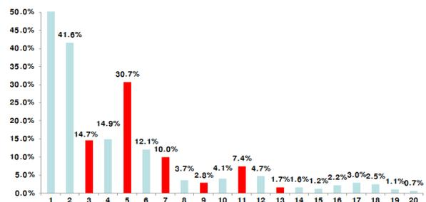
Figure 1: Current spectrum of the input electric power of the CCPS.
