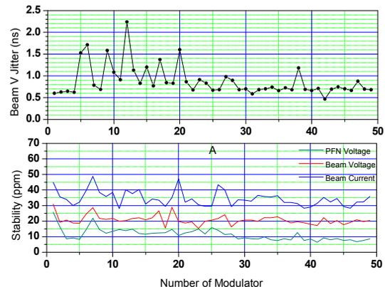
Figure 2: PFN voltage (green), measured stabilities of beam voltage (red) and beam current (blue), and timing jitter of beam voltage.
