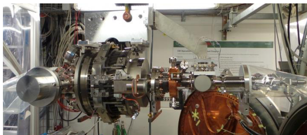
Figure 2: Coaxial tuner with quad piezos assembled to the gun cavity at HZB [3].
