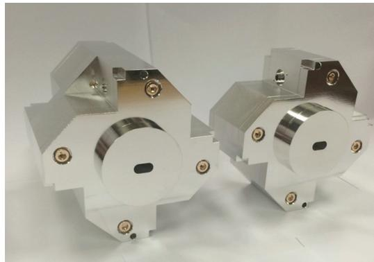
Figure 1: The fabricated low-Q IPBPM.
