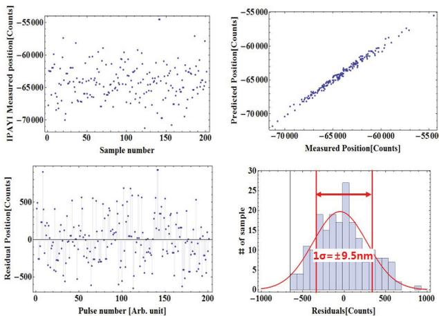
Figure 5: The measured position resolution of IPBPM-A is 9.5nm with  $0.869 \times 1.6\text{nC}$  beam charge condition.
