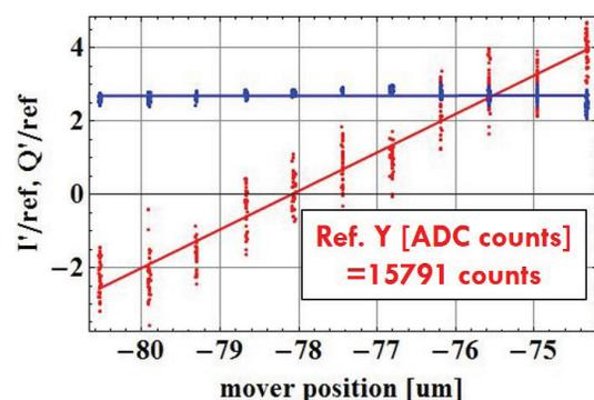
Figure 4: Low-Q IPBPM-A calibration factor. Normalized I' signal (Red) and normalized Q' signal(Blue).
