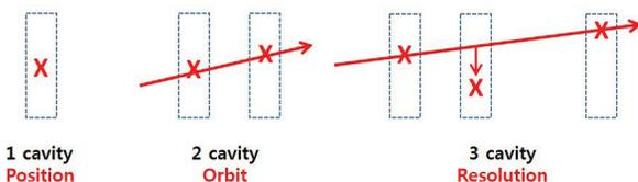
Figure 3: The principle of beam position resolution measurement of IPBPM.
