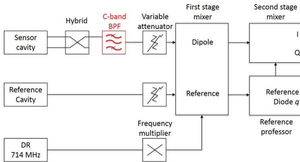
Figure 2: The beam test scheme of low-Q IPBPM entire system.
