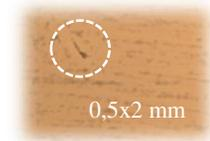
Figure 2. Example of shrinkage defect in copper, seen on IPHI RFQ after machining.
