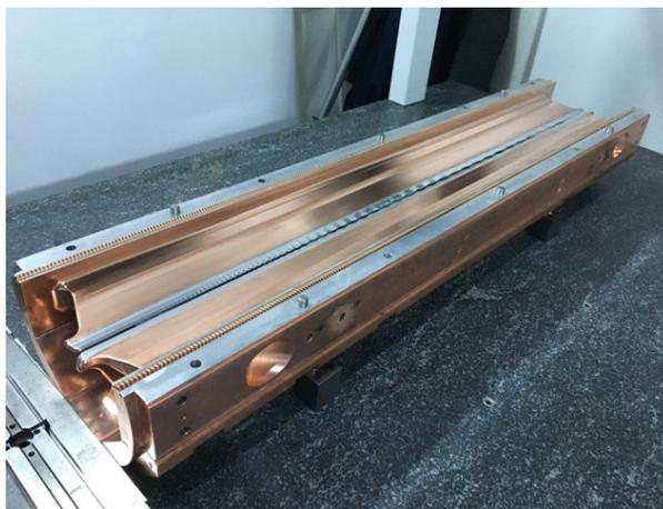
Figure 4: Assembling of the vanes.
