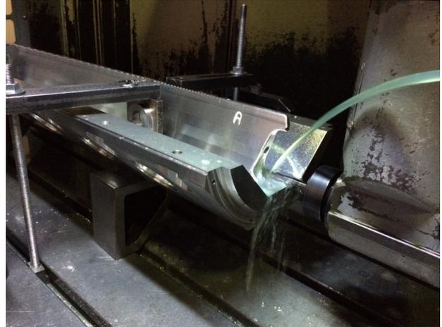
Figure 1: Machining of the cut-backs.
