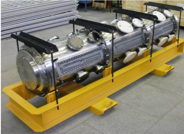
Figure 2: New RFQ resonator before coppering.
