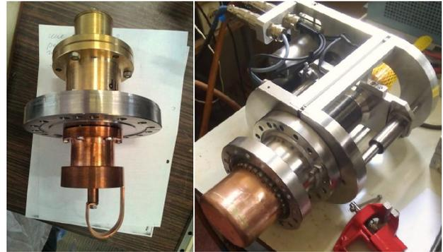
Figure 5: RF coupling loop (left) and tuning plunger.
