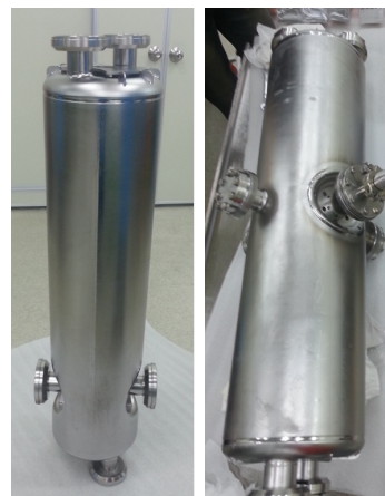
Figure 3: Quarter wave resonator and half wave resonator after final electron beam welding.
