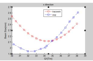
Figure 2: beam spot size in x direction, where the blue points are experiment data, and the red ones are gotten with Partran of TraceWin. During tracking, the Twiss parameters from traditional method are used.
