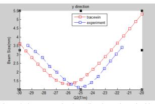
Figure 3: beam spot size in y direction, where the blue points are experiment data, and the red ones are gotten with Partran of TraceWin. During tracking, the Twiss parameters from traditional method are used.
