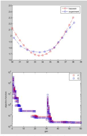
Figure 5: beam size data in y direction from experiment and simulation with 'Partran' code. The input Twiss parameters are from MOGA.
