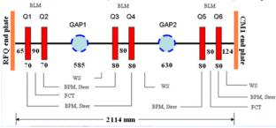
Figure 1: The lattice and diagnostic element layout of MEBT1 in CADS injector I.
