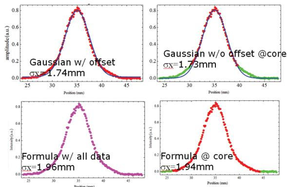
Figure 2: Fitting results for a quasi-gaussian signal with four different fitting methods. The green dots shown in the right plots are excluded in the fitting or calculation of beam sizes.
