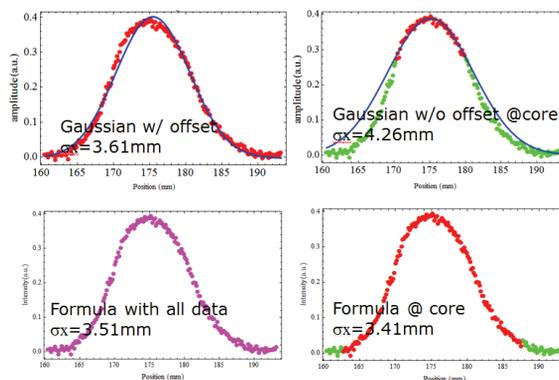
Figure 4: Fitting results for a wide-plump signal with four different fitting methods. The green dots shown in the right plots are excluded in the fitting or calculation of beam sizes.
