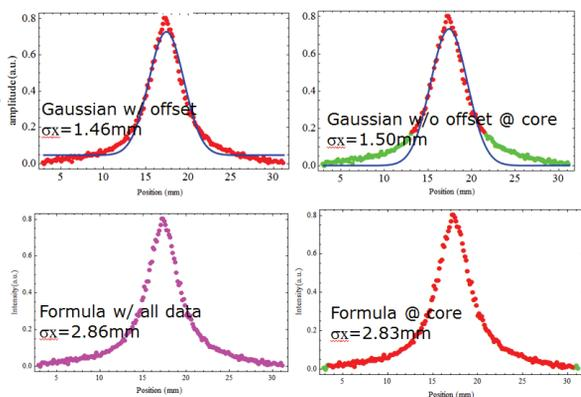
Figure 3: Fitting results for a narrow-pointed signal with four different fitting methods. The green dots shown in the right plots are excluded in the fitting or calculation of beam sizes.
