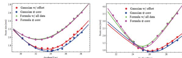
Figure 5: Fitting results of beam emittances at horizontal (left) and vertical (right) planes. The dots are beam sizes obtained with four different fitting methods, and the lines are the beam sizes calculated with the fitted TWISS parameters and emittances using the corresponding beam sizes set.
