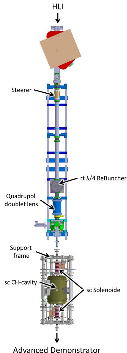
Figure 1: Top view of the construction layout of the cw-LINAC demonstrator section comprising rt  $\lambda/4$  re-buncher cavity and the cryostat; the sc CH-cavity is surrounded by two sc solenoids on a support frame (cryostat is not shown).
