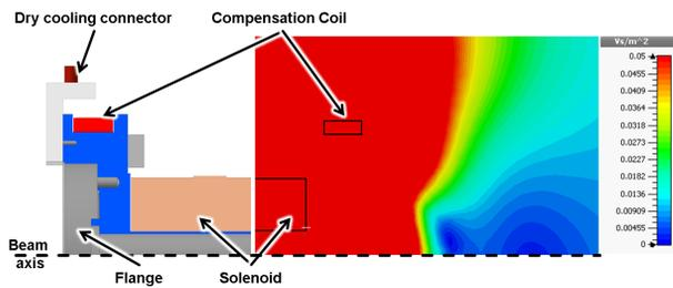
Figure 5: Cross sectional view (left) and a typical example of the magnetic field distribution of the solenoid with compensation coils (right).
