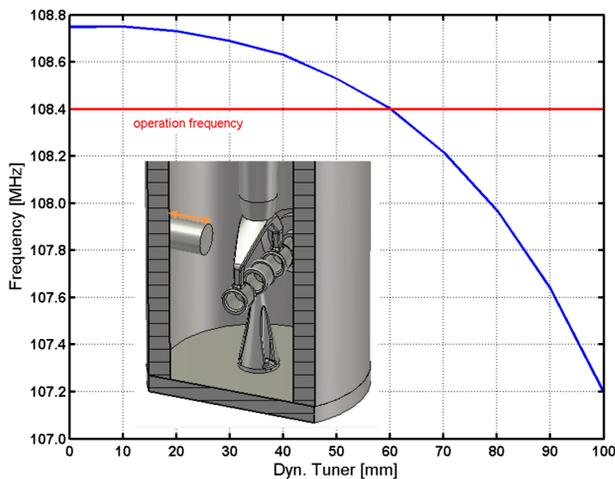
Figure 3: Simulated frequency range of the  $\lambda/4$  rebuncher depending on the position of the dynamical plunger. The plunger (radius: 25 mm) has a length of 60 mm in operation.
