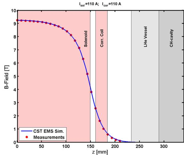
Figure 6: Simulated and measured magnetic field in the cavity region of the sc solenoid with compensation coils.
