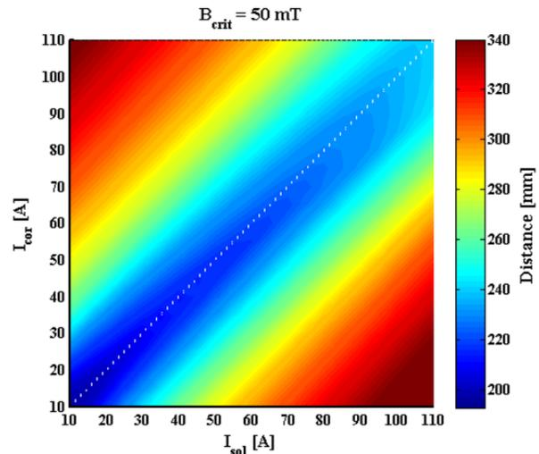
Figure 7: Minimum Distance  $z$  (color) at  $B_{crit} = 50$  mT for all current combinations of the solenoid ( $I_{sol}$ ) and the compensation coils ( $I_{cor}$ ).
