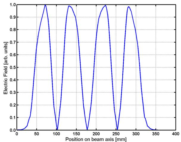
Figure 4: Simulated electrical field distribution on beam axis at 108.4 MHz for the  $\lambda/4$  rebuncher.
