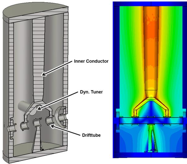
Figure 2: Cross sectional view (left) and magnetic field distribution (right) of the four gap  $\lambda/4$ -re-buncher; the dynamical plunger is shown in the background; the drift tubes are equipped with bulges to reduce the dipole effect.
