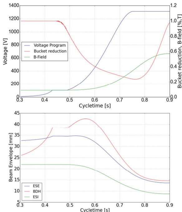
Figure 6: Optimised voltage program and bucket reduction factor for a 252.7MeV cycle and a ramp rate of 2.2T/s (top). Evolution of beam envelope (bottom) at electrostatic extraction and injection septum (ESE/ESI) and horizontal beam dump (BDH).
