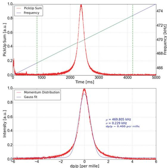
Figure 3: Empty Bucket scan on a coasting beam after synchrotron injection. Frequency sweep with envelope of BPM sum signal (top) and momentum distribution (bottom).
