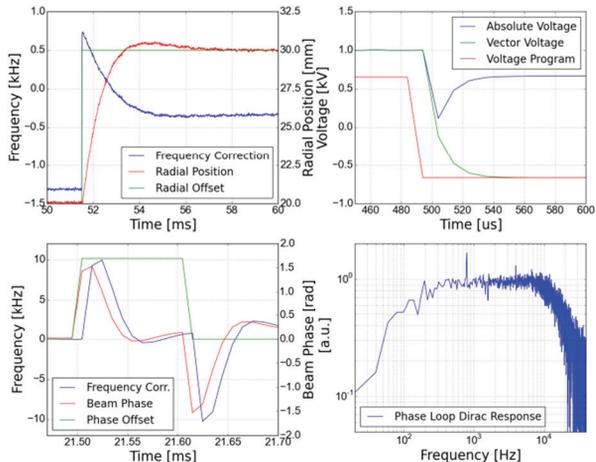
Figure 2: Step response of the radial loop (top left), voltage loop (top right), double step (lower left) and Dirac impulse response (lower right) of phase loop.
