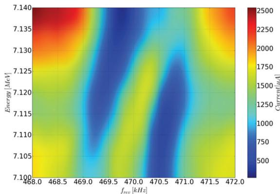
Figure 5: Varying the main ring dipole field at injection in terms of energy equivalent and the capture frequency reveals the local particle current optimum at 470kHz and 7.125MeV.
