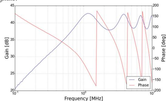
Figure 1: Transfer function of the amplifier-cavity ensemble used for the LLRF compensation table.
