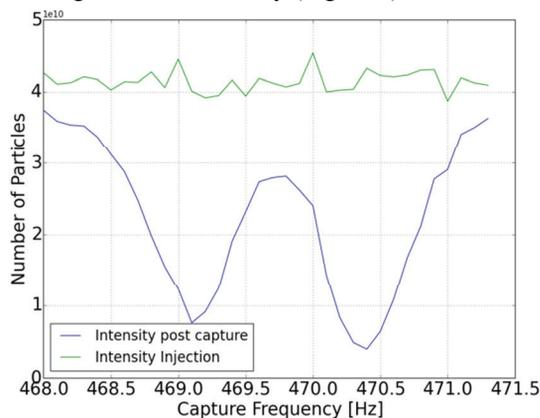
Figure 4: Typical injection frequency scan for adiabatic capture with a 106V bucket and a 0.05 adiabaticity. The plot shows the initial intensity after injection and the remaining intensity after capture.
