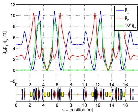
Figure 2: ThomX storage ring nominal optics: horizontal beta function (blue), vertical beta function (red), and horizontal dispersion (green).
