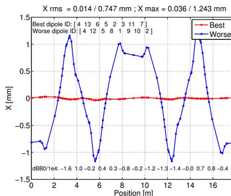
Figure 4: Dipole sorting procedure on the ThomX SR assuming Gaussian error distribution with  $(\text{dB}/\text{B})_{\text{rms}}=1/10^4$ . Best and worse case of the closed orbit distortion.
