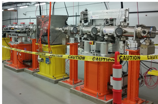
Figure 3: Both dechirper modules as installed in the SLAC LCLS. Between the two modules is a quadrupole magnet.
