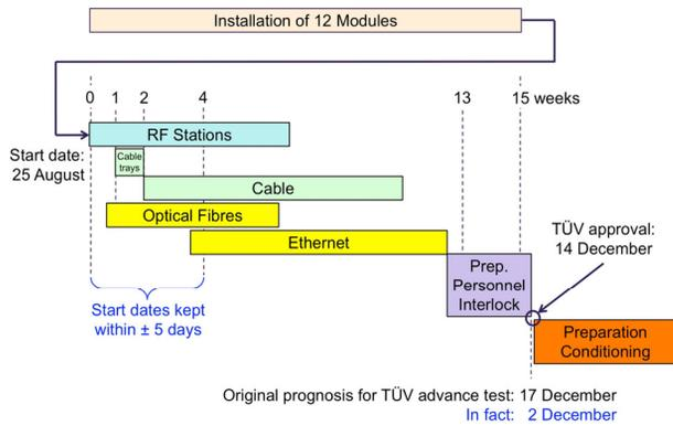
Figure 4: First installation process, according to the newly developed plan, finishes two weeks earlier than expected.
