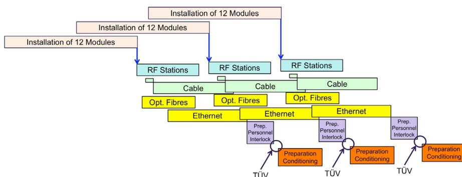
Figure 2: Installation sequence of several accelerator sections (so called cryo-strings including 12 modules) in a Gantt diagram. Each block represents 4 to 24 installation steps.
