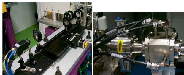
Figure 3: Left : Optical setup for imagers. Right: ICT 2 (left) and cBPM 2 (right) at the exit of the undulator.
