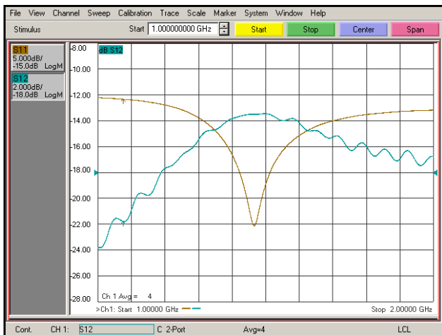
Figure 4: Testing results of the prototype device. The coupling is best at 1.47 GHz (minimum S11, yellow) and at that frequency, S12 is -13.54 dB which is very close to the simulated value of -13.222 dB.
