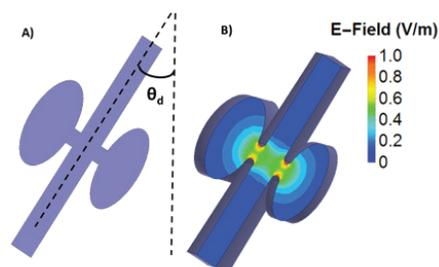
Figure 1: An image of (A) general cross section of a typical output cavity at angle  $\theta_d$  as it relates to the deflection angle of the e-beam and (B) a contour plot of the electric field for the TM mode of operation.
