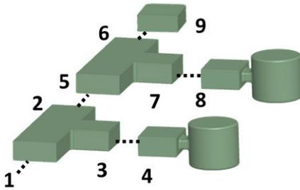
Figure 3: The 9-port (1 external) power extraction network featuring two isolated resonators at arbitrary frequency, phase, and power.
