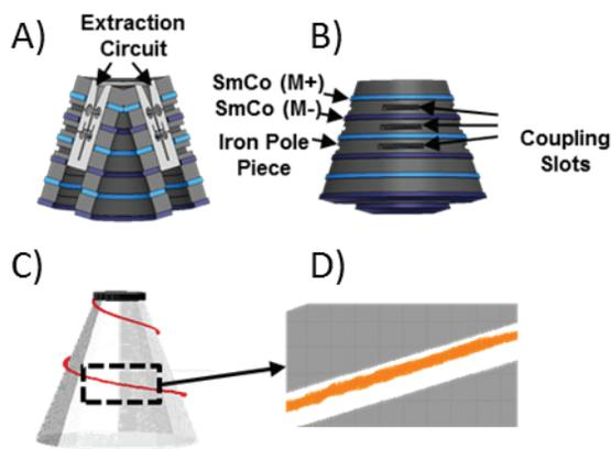
Figure 4: An image of (A) a cross section of the PPM array on the exterior of the extraction network, (B) the external rendering of the PPM array with coupling slots, (C) a MAGIC PIC simulated deflecting beam with PPM fields, and (D) an enlarged image of the beam inside the drift tube.
