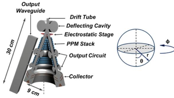
Figure 2: A 3-D CAD rendering of the DBA conceptual configuration at S-band.
