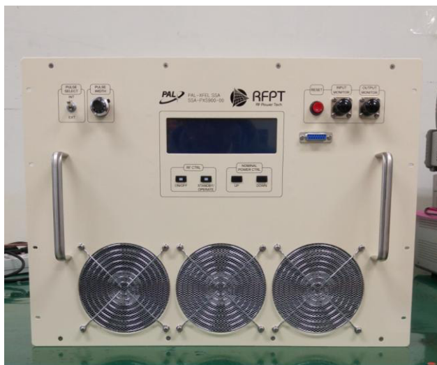
Figure 7: Photograph of the 1 kW X-band SSA to drive the X-band klystron.
