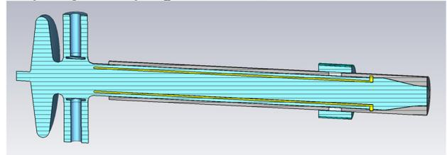
Figure 1: Coaxial HOM damping design of the 704 MHz SRF booster cavity.
