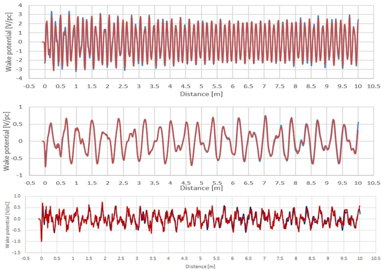
Figure 2: Single bunch wake potential in 10m for a) 2.1 GHz warm cavity (top); b) 704 MHz warm cavity (middle); c) 704 MHz booster SRF cavity (bottom). Blue curves are from the reconstruction of Eigen mode simulation, and red curves are from CST Particle Studio™.
