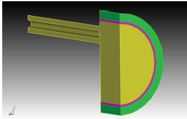
Figure 1: A cartoon of the interior of the high pressure test cell (including coupler). The volume filled with nitrogen gas (green and yellow) and alumina tube (magenta) are shown.
