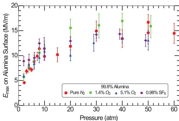
Figure 5: Maximum electric field on the surface of the 99.8% alumina torus as a function of gas pressure for pure nitrogen, and nitrogen doped with oxygen or sulfur hexafluoride. The error bars represent the statistical uncertainty.
