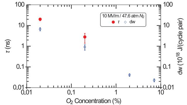
Figure 4: Attachment time of electrons to oxygen molecules and energy dissipation per charged particle pair per RF cycle as a function of oxygen concentration. The error bars represent the systematic uncertainty for  $\tau$ , and the statistical and systematic uncertainty for  $dw$ .
