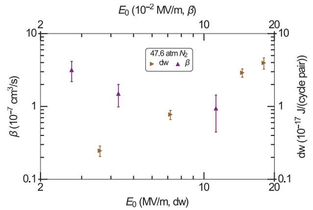
Figure 3: Recombination rate of electrons with nitrogen ions and energy dissipation per charged particle pair per RF cycle as a function of electric field amplitude. The error bars represent the statistical uncertainty for  $\beta$ , and the statistical and systematic uncertainty for  $dw$ .
