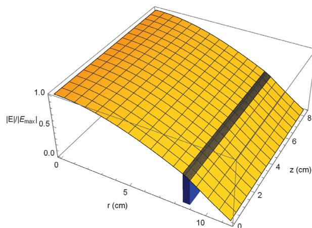
Figure 2: Normalized electric field distribution for the high pressure test cell loaded with an alumina tube. The shaded blue region indicates the area the alumina occupies.
