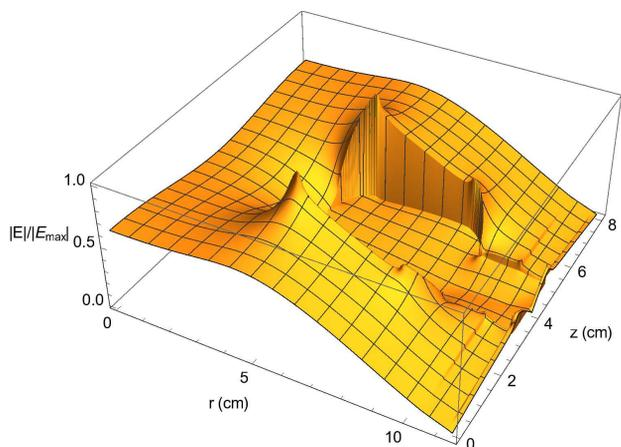
Figure 2: Electric field map for the dielectric loaded high pressure test cell. The plot has been normalized to the maximum electric field, which occurs at the interior rounded surface of the alumina.
