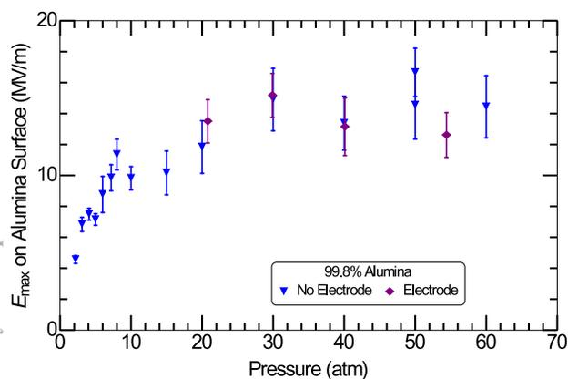
Figure 5: Electric field on the surface of the alumina torus at which sparking occurred as a function of pure nitrogen gas pressure. The cases of with and without the copper electrodes are shown. The error bars represent the standard deviation of the measurements.
