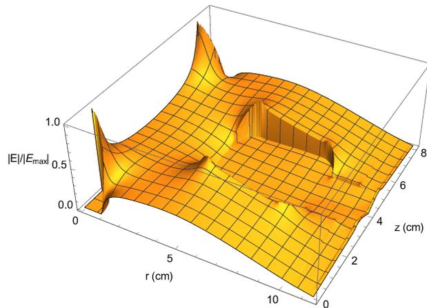
Figure 4: Electric field map for the dielectric loaded high pressure test cell. The plot has been normalized to the maximum electric field, which occurs at the tip of the copper electrodes.
