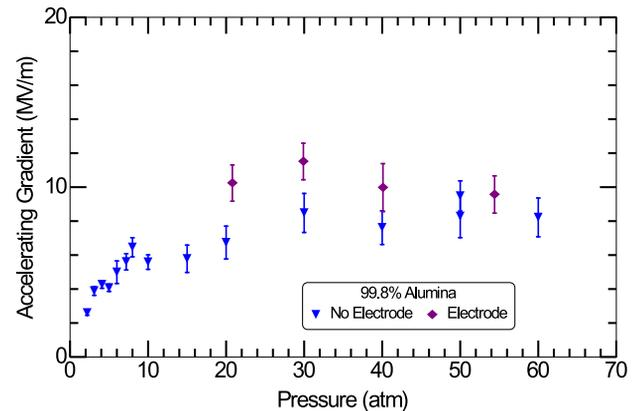
Figure 6: Average accelerating gradient at which sparking occurred as a function of pure nitrogen gas pressure. The cases of with and without the copper electrodes are shown. The error bars represent the standard deviation of the measurements.
