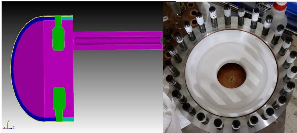
Figure 1: The high pressure test cell with an alumina torus and teflon spacers. On the left is a cartoon of the interior of the cavity (including coupler) in which the nitrogen gas (magenta and yellow), alumina torus (green), and teflon spacers (blue and teal) are shown. On the right is a photo of the interior of the cavity with one end plate removed. The alumina torus and one teflon spacer are visible, as well as the copper plug (on axis), clamping bolts, and one of two RF and pressure seals.
