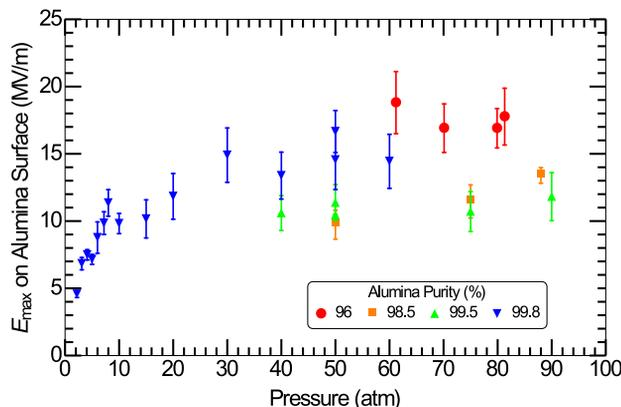
Figure 3: Electric field on the surface of the alumina torus at which sparking occurred as a function of pure nitrogen gas pressure. The error bars represent the standard deviation of the measurements.
