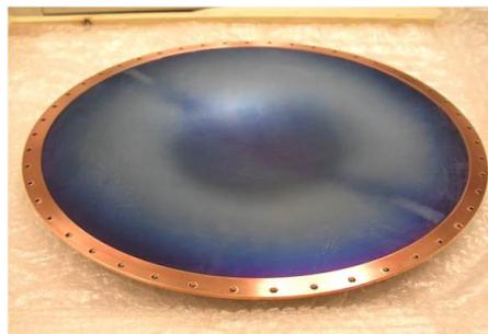
Figure 1: Beryllium window for MICE cavity, with 0.38 mm thickness, 42 cm diameter and about 18 mm depth of the bow.
