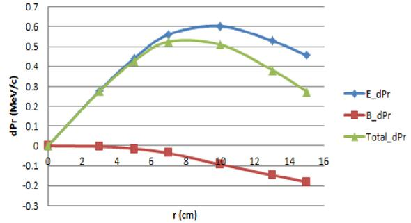
Figure 5: The transverse kick on a 200 MeV/c muon beam due to E field, B field and the total kick, normalized to 10 MV longitudinal acceleration.
