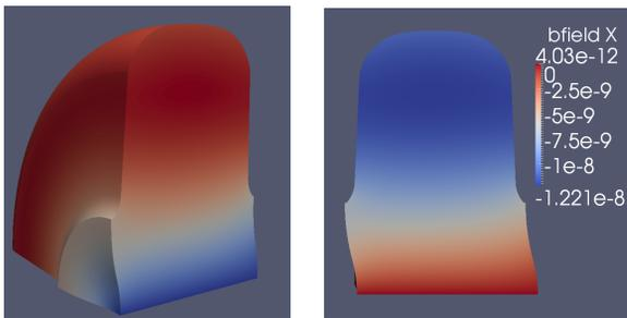
Figure 4: Magnetic field solved by Omega3P: left the B field magnitude, right the B field azimuthal component.
