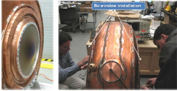
Figure 2: Installed Be window on MICE cavity (left) and Be window installation (right).
