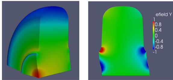
Figure 3: Electric field solved by Omega3P: left the E field magnitude, right the E field transverse component.
