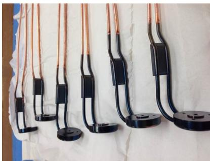
Figure 4: TiN coating of the coupling loop
