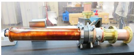
Figure 5: The assembled RF coupler
