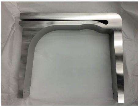
Figure 8: Tuner arm after UHV cleaning.
