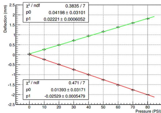
Figure 9: Actuator functional test: Deflection vs Applied pressure.
