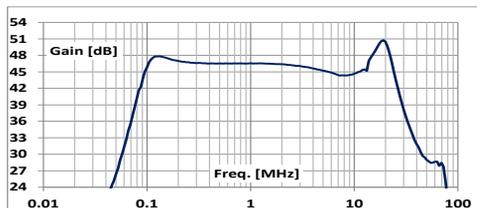
Figure 3: Cell frequency response.
