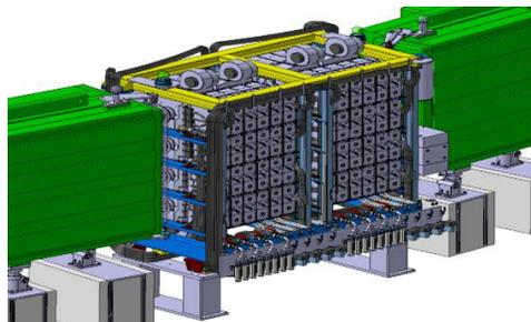
Figure 2: Group of four superimposed couples of cavities in one PSB Section.
