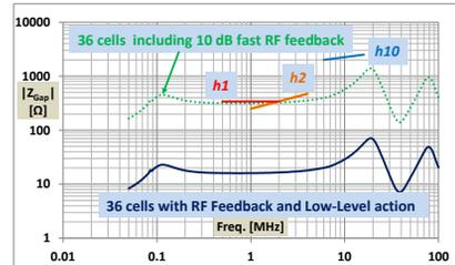
Figure 6: Overall impedance as seen by the beam. *h1*, *h2* and *h10* are the impedances of the system being replaced.
