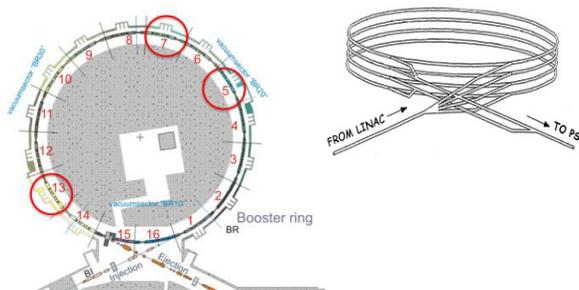
Figure 1: Cavities position in the PSB ring.
