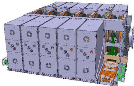
Figure 5: 6-cell cavity with amplifiers assembly.
