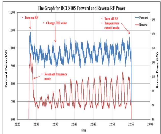
Figure 6: The graph for RCCS105 RF power.
