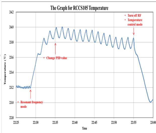
Figure 3: The graph for RCCS105 temperature.
