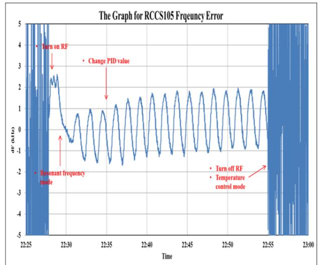
Figure 5: The graph for RCCS105 error frequency.
