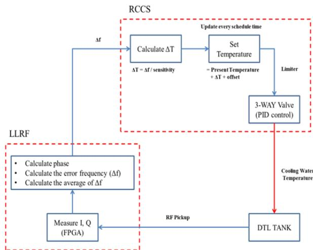
Figure 2: Block diagram of the resonant frequency control mode.
